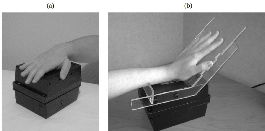
Figure 2: (a) Hand positioning on the device during palmar vascular pattern image acquisition; (b) additional set-up and hand positioning during wrist vascular pattern image acquisition
